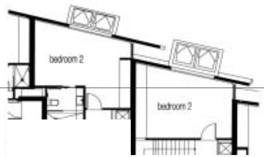
Part plan of Building 2 showing the staggered precast walls to the upper level bedrooms
