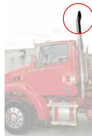
Figure 2 Exhaust vented above cabin height
