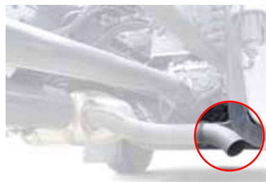
Figure 1 Exhaust Location Standard Euro V Truck Specification
