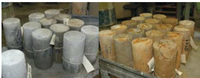
Plate 3 Cylinders after 3 years exposure prior to compression test. Grey in neutral sulfate solution ( left ). Rustic red in acidic sulfate solution ( right )
